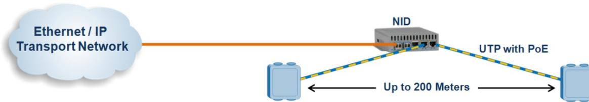
Figure 3 – NID with Power over Ethernet
