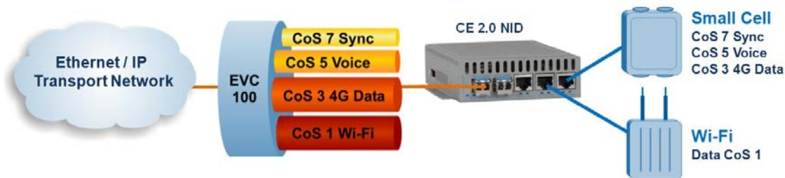
Figure 1 – Carrier Ethernet 2.0 Multi-CoS Performance Monitoring
