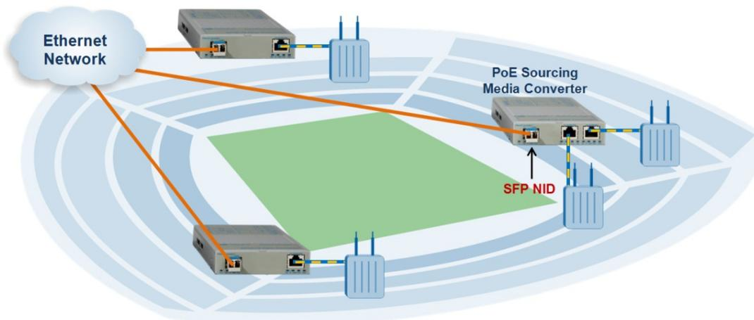
Figure 4 – Carrier Ethernet Backhaul with PoE Media Converters + SFP NIDs
