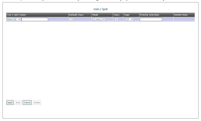
Class of Service (CoS) is supported by mapping customer frames into eight egress queues based on using the 3-bit Priority Code Point (PCP) field in the VLAN tag.
