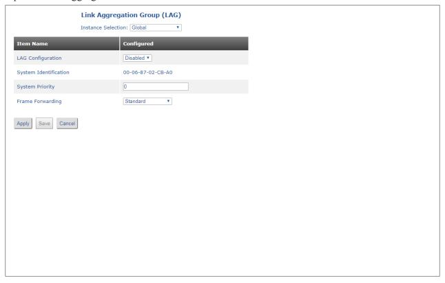
Link Aggregation Groups (LAG) and Link Aggregation Control Protocol (LACP) are methods to provide more than one link between two devices and automate the configuration and maintenance of the links. LAG and LACP is defined in the IEEE 802.1ax standard.
