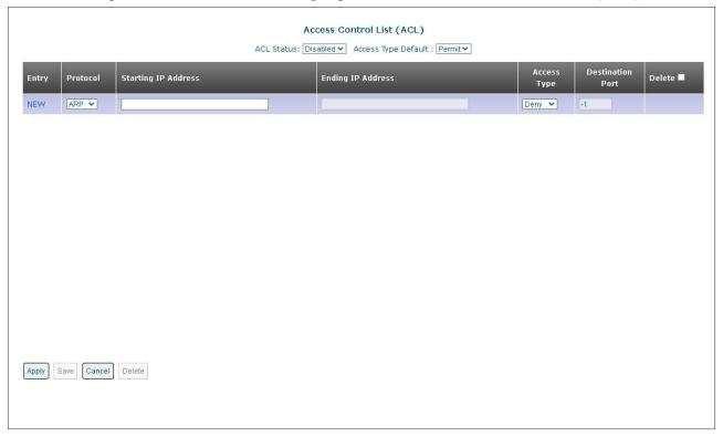
Access Control Lists can prevent certain traffic from entering or exiting the management port. ACLs can be configured for ARP, ICMP, IP, TCP and UDP protocols. These protocols can be configured to be permitted or denied access.
