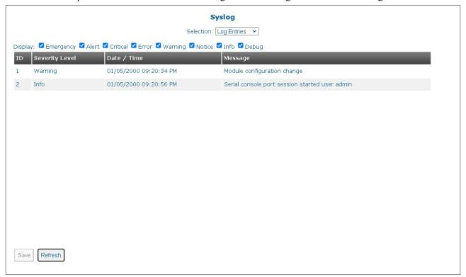
Check the boxes of the severity level to be displayed in the log.
