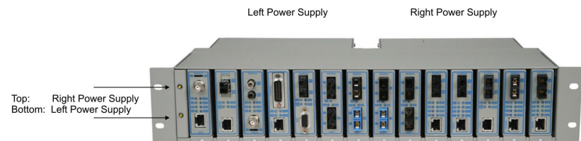
14-Module Chassis Showing Power Supply Location and Power LEDs
